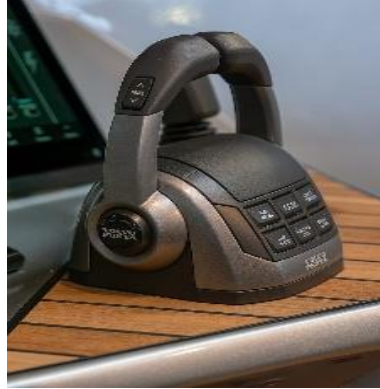
Dual engine control levers by Volvo Penta Marine of a SAY 42 carbon yacht
